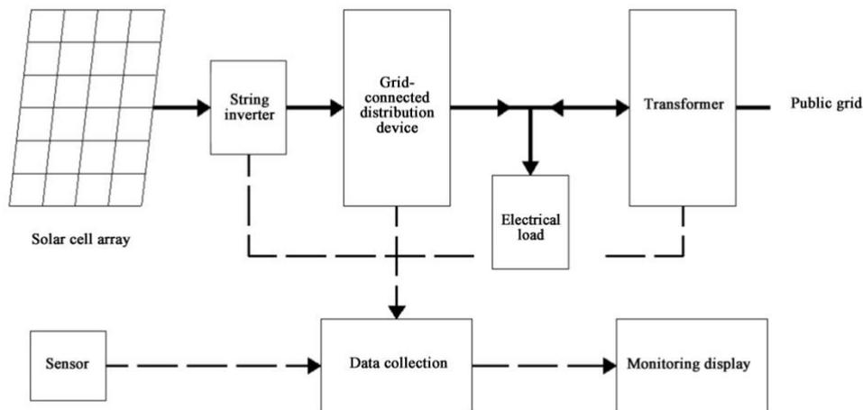
Figure 2.5-1 Schematic Diagram of Grid-connected PV Power Generation
